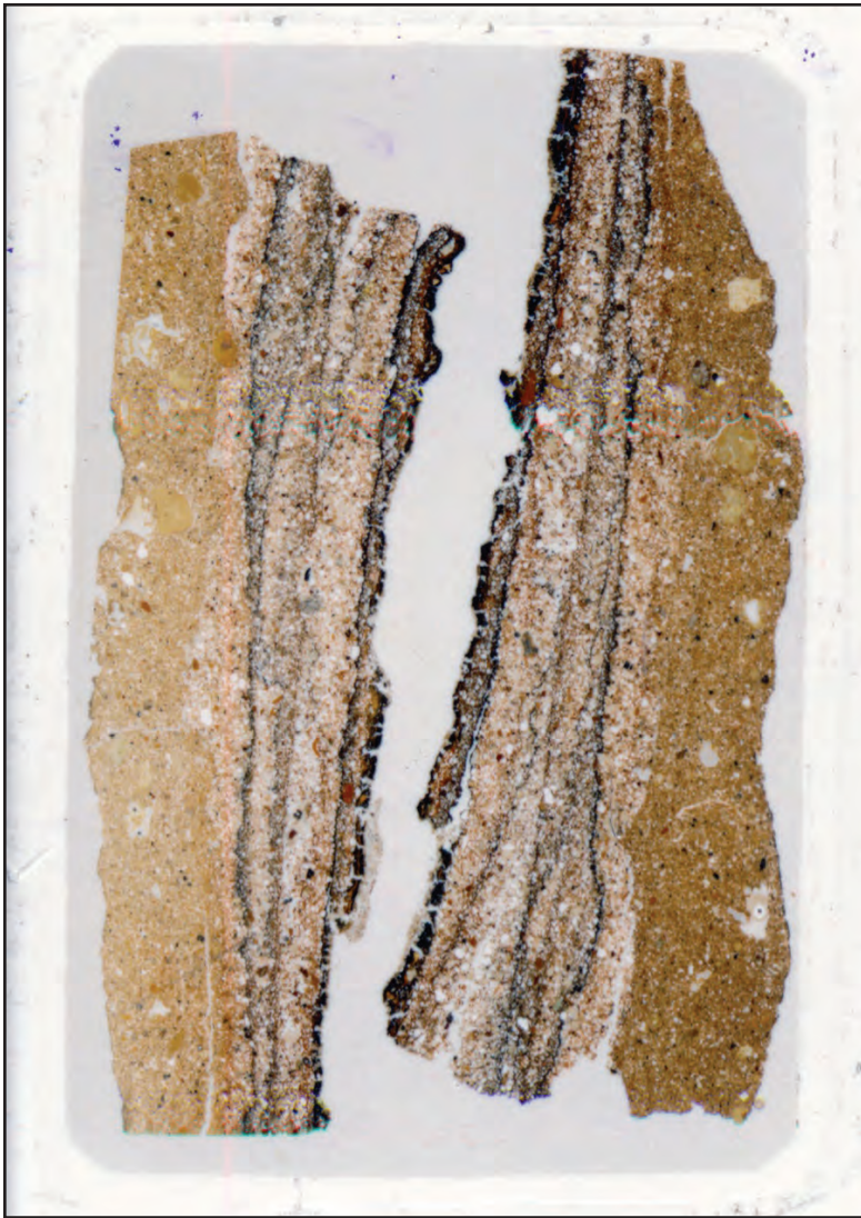
Figure 3. Thin section of finish plaster in Room 3-4, south wall, showing up to six plaster and wash layers separated by dust and soot
